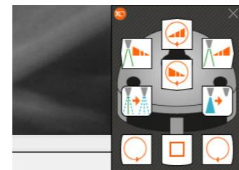
Set instrument parameters for each treatment e.g. speed, speed curve, torque limit or the amount of water and air.
